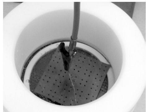
Figure 10 – Cross-section and photograph of anodization cell. Not shown in the cross section is a secondary piece which screws down into the outside holder, producing downward force that seals the top of the cell (the HF side) from the bottom of the cell.
